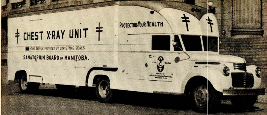
In one day, 1,250 people can be X-rayed by this 70mm mobile unit, using movie-type film.
