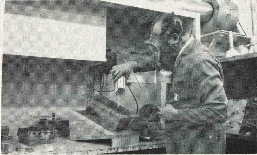
At the Winnipeg Pattern and Model Works, where SACH feet are now made, Steve Buchko loads a mold with polyurethane foam rubber.
